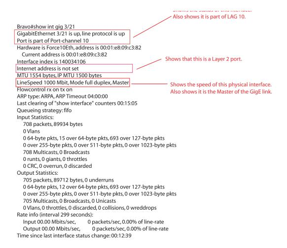
Using the show interfaces port-channel Command to Inspect LAG 10
