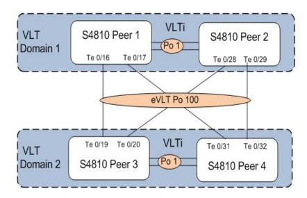
In Domain 1, configure Peer 1 fist, then configure Peer 2. When that is complete, perform the same steps for the peer nodes in Domain 2. The interface used in this example is TenGigabitEthernet.
