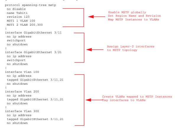
Figure 30-135. SFTOS Example Running-Configuration
