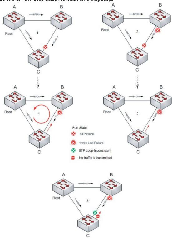
Figure 48-343. STP Loop Guard Prevents Forwarding Loops
