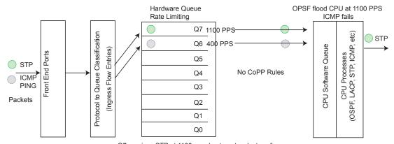
Q7 receives STP at 1100 pps due to network storm/loop.
