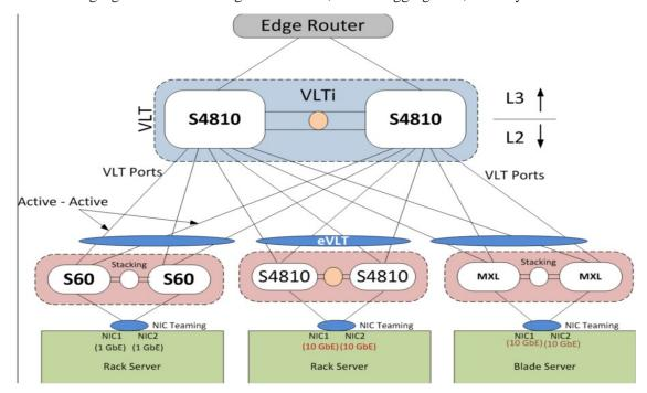
The aggregation layer is mostly in the L2/L3 switching/routing layer. For better resiliency in the aggregation, Dell Force10 recommends running the Internal Gateway Protocol on the VLTi VLAN to synchronize the L3 routing table across the two nodes on a VLT system.
