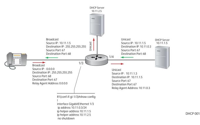
To view the **ip helper-address** configuration for an interface, use the command **show ip interface** from EXEC privilege mode, as shown in the following example.
