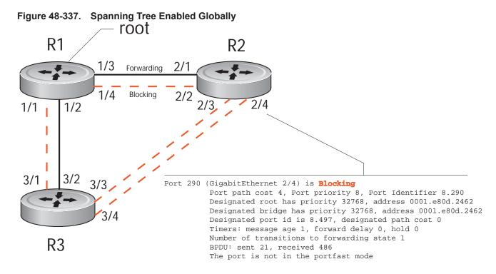
View the Spanning Tree configuration and the interfaces that are participating in STP using the show spanning-tree 0 command from EXEC privilege mode. If a physical interface is part of a port channel, only the port channel is listed in the command output.
