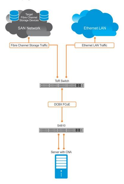
The following sections describe how to configure the FIP snooping feature on a switch that functions as a FIP snooping bridge so that it can perform the following functions:
