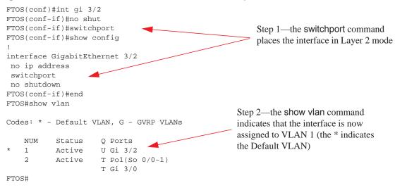
By default, VLAN 1 is the Default VLAN. To change that designation, use the default vlan-id command in the CONFIGURATION mode. You cannot delete the Default VLAN.
