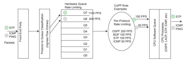
CoPP restricts the STP control packet rate to the CPU to 100 pps. PING works reliably.
