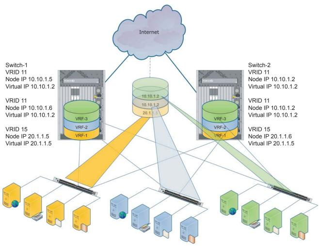
Figure 54-397 shows a typical use case in which three virtualized overlay networks are created by configuring three VRFs in two E-Series switches. The default gateway to reach the internet in each VRF is a static route with the next hop being the virtual IP address configured in VRRP. In this scenario, a single VLAN is associated with each VRF.
