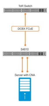
In Figure 16-37, DCBX and PFC are enabled on the FIP snooping bridge and on the FCF ToR switch. On the FIP snooping bridge, DCBX is configured as follows:
