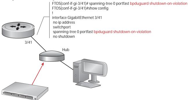
Switch with Spanning Tree Enabled
