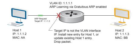
Whether ARP Learning via Gratuitous ARP is enabled or disabled, the system does not look up the Target IP. It only updates the ARP entry for the Layer 3 interface with the source IP of the request.
