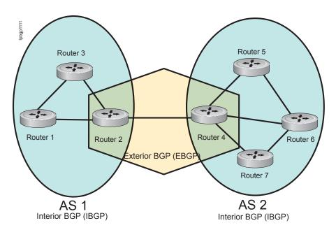
BGP version 4 (BGPv4) supports classless interdomain routing and aggregate routes and AS paths. BGP is a path vector protocol - a computer network in which BGP maintains the path that update information takes as it diffuses through the network. Updates traveling through the network and returning to the same node are easily detected and discarded.
