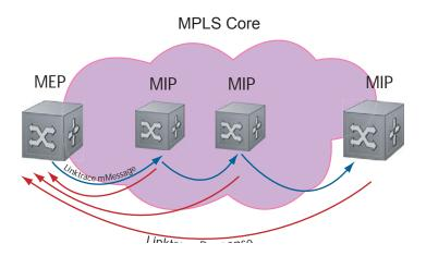
Link trace messages carry a unicast target address (the MAC address of an MIP or MEP) inside a multicast frame. The destination group address is based on the MD level of the transmitting MEP (01:80:C2:00:00:3[8 to F]). The MPs on the path to the target MAC address reply to the LTM with an LTR, and relays the LTM towards the target MAC until the target MAC is reached or TTL equals 0.
