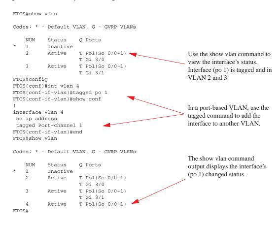
Except for hybrid ports, only a tagged interface can be a member of multiple VLANs. Hybrid ports can be assigned to two VLANs if the port is untagged in one VLAN and tagged in all others.
