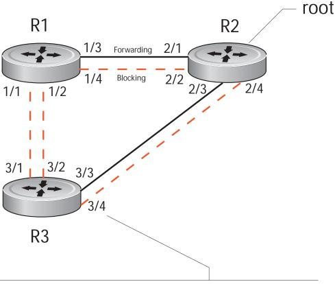
Port 684 (GigabitEthernet 4/43) is alternate Discarding Port path cost 20000, Port priority 128, Port Identifier 128.684 Designated root has priority 32768, address 0001.e801.cbb4 Designated bridge has priority 32768, address 0001.e801.cbb4 Designated port id is 128.684, designated path cost 20000 Number of transitions to forwarding state 0BPDU : sent 3, received 219 The port is not in the Edge port mode
