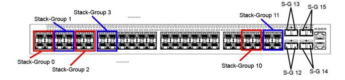
You can connect the units while they are powered down or up. Stacking ports are bi-directional.
