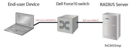
The illustration above and the illustration below show how EAP frames are encapsulated in Ethernet and RADIUS frames.
