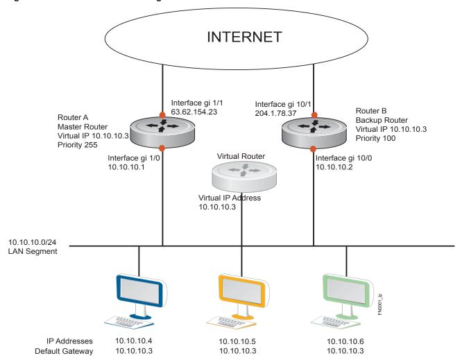
For more detailed information on VRRP, refer to RFC 2338, Virtual Router Redundancy Protocol.
