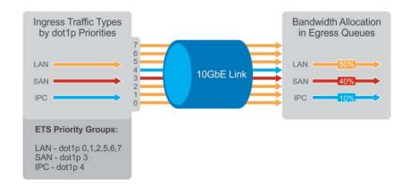
Figure 13-6. Enhanced Transmission Selection
