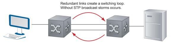
Use backup interfaces to create redundant links in networks without STP
