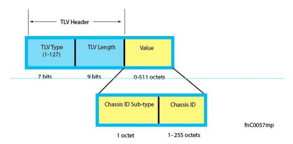
TLVs are encapsulated in a frame called an LLDP Data Unit (LLDPDU) (Figure 28-83), which is transmitted from one LLDP-enabled device to its LLDP-enabled neighbors. LLDP is a one-way protocol. LLDP-enabled devices (LLDP agents) can transmit and/or receive advertisements, but they cannot solicit and do not respond to advertisements.
