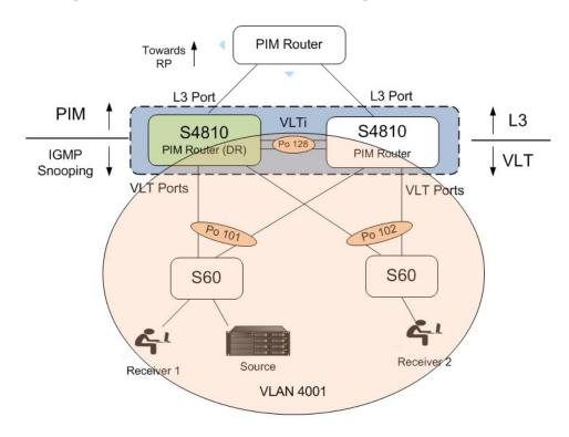
On each VLAN where the VLT peer nodes act as the first hop or last hop routers, one of the VLT peer nodes will be elected as the PIM Designated Router. If IGMP Snooping is configured along with PIM on the VLT VLANs, then VLTi must be configured as the static multicast router port on both VLT peer switches. This allows multicast traffic that originates from the source that is connected to the VLT ports to reach the PIM router which has downstream neighbors.
