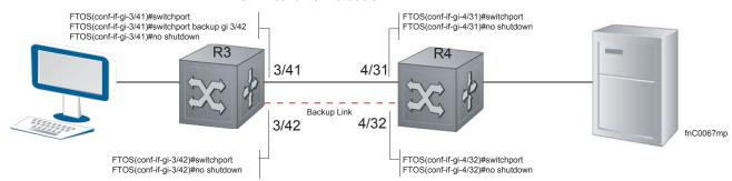
You configure a redundant pair by assigning a backup interface to a primary interface with the switchport backup interface command. Initially, the primary interface is active and transmits traffic and the backup interface remains down. If the primary fails for any reason, the backup transitions to an active UP state. If the primary interface fails and later comes back up, it remains as the backup interface for the redundant pair.
