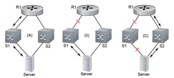
A: Switches1 and 2 have upstream and downstream connections to Router1 and Server via primary links. B: Upstream link between Switch1 and Router1 fails. Downstream link with Server stays up temporarily. C: Switch1 disables downstream link to Server. Server starts to connect with Router1 using backup link to Switch2; Switch2 starts to use the backup link to Router1.
