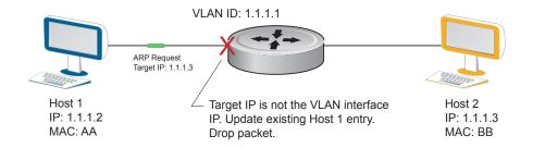
Beginning with FTOS version 8.3.1.0, when ARP Learning via Gratuitous ARP is enabled, the system installs a new ARP entry, or updates an existing entry for all received ARP requests.
