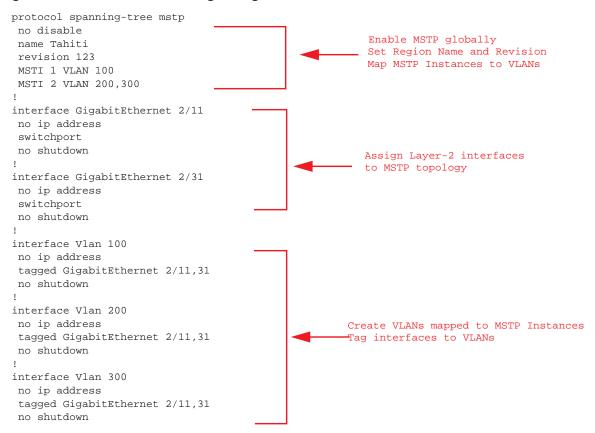
Figure 30-134. Router 3 Running-configuration
